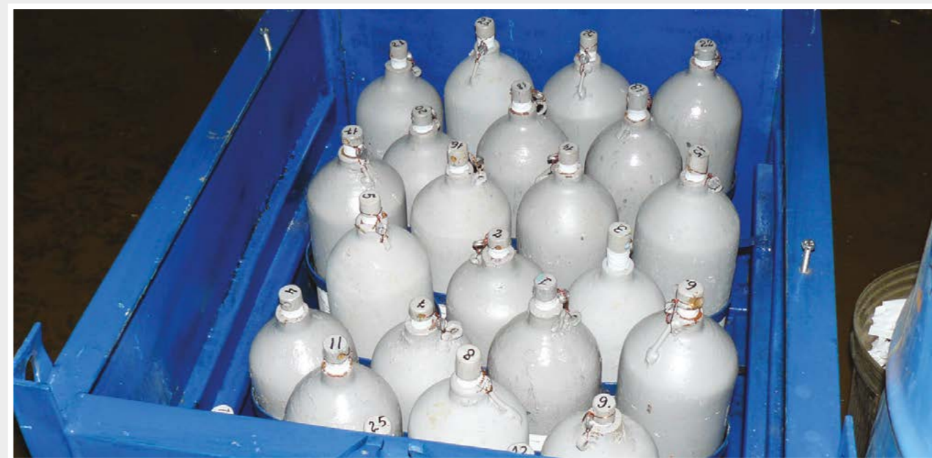
Container for transportation of mercury ©Mercom Ltd
